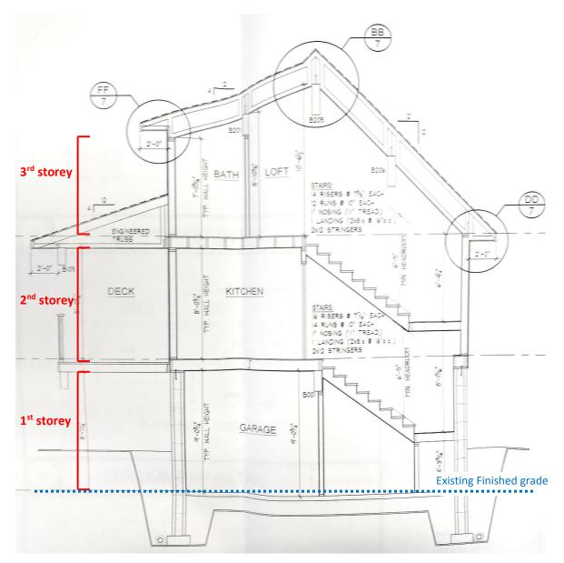
The submitted plans show the garage and habitable space to be at grade. The entry level is classified as the 1<sup>st</sup> storey with the 2<sup>nd</sup> and 3<sup>rd</sup> storeys above. A Development Variance Permit is needed to allow the third storey.
