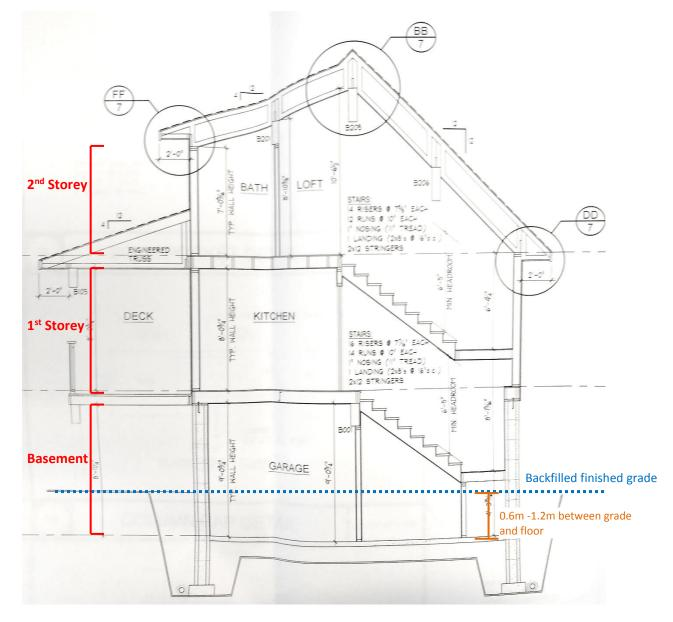
Labelling of floor levels, if the entry floor is sunk 0.6m – 1.2m below the finished grade
