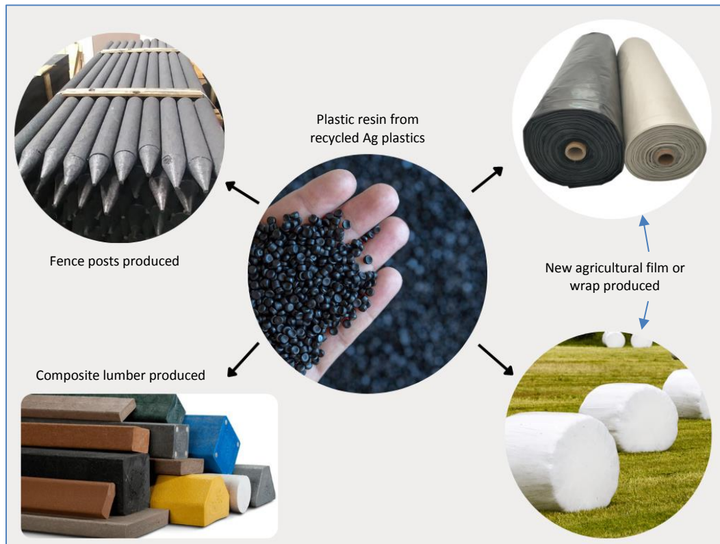
Figure 1. Plastic resin from Ag plastics can be made into plastic fence posts, composite lumber, or new agricultural film, among other items.
