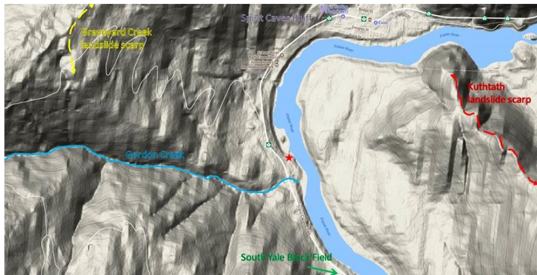
FIGURE 5: LARGE FAILURES IN THE AREA. SOUTH YALE BLOCKFIELD AND SPIRIT CAVES BLUFFS ARE OFF THE IMAGE BUT GENERAL DIRECTION IS INDICATED. PROPERTY LOCATED AT RED STAR IN CENTER OF IMAGE. ALL LOCATIONS ARE APPROXIMATE.
