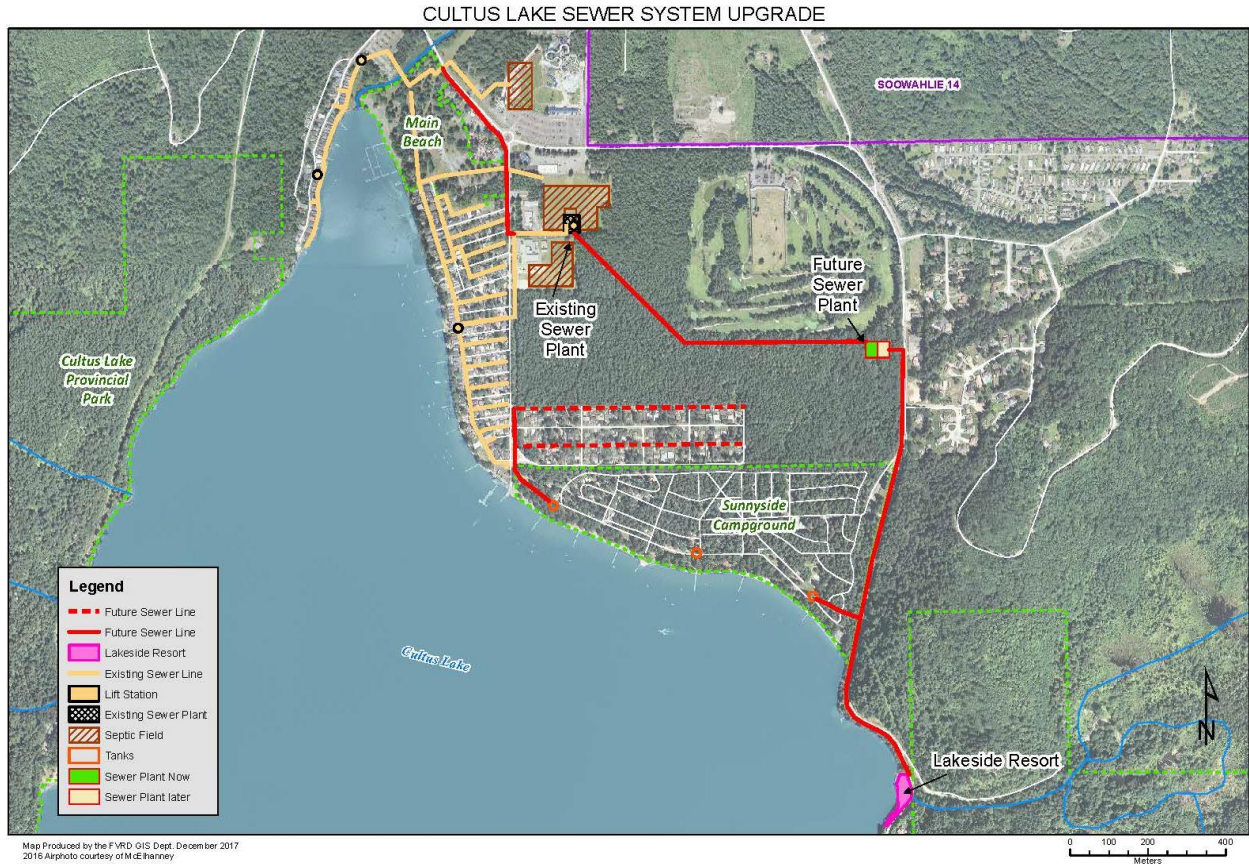
Figure 1: Existing and Future Sewer System Locations
