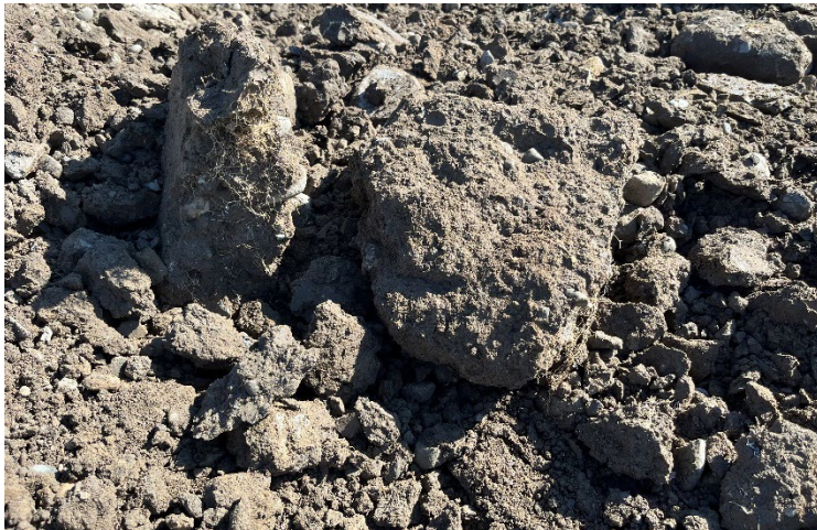
Figure 9. Photo showing some larger rocks and pieces of concrete in the imported fill.
