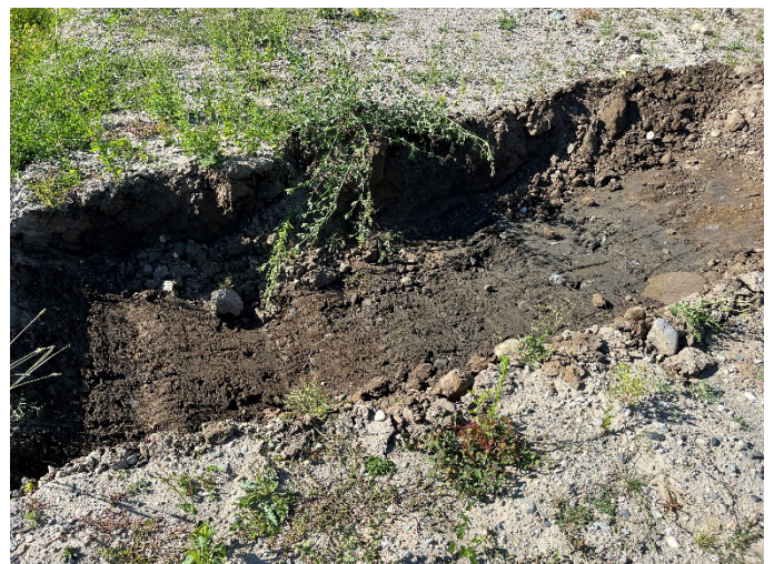
Figure 12. Photo showing the depth of fill and that most of the fill was free of debris.
