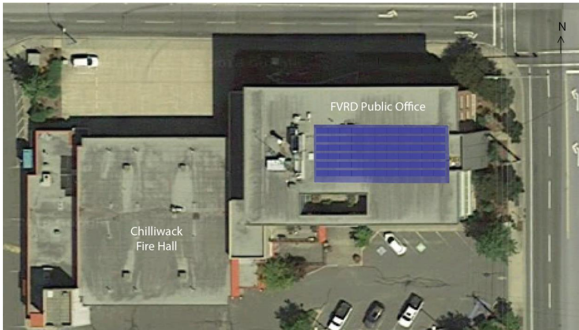
Figure 1: Footprint of the 22.7 kW Solar Panel Array on FVRD office roof.
