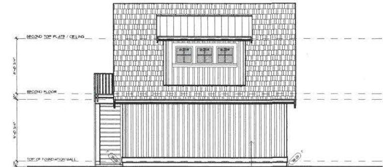
DETACHED GARAGE WEST ELEVATION SCALE: 1/4" = 1'-0"
