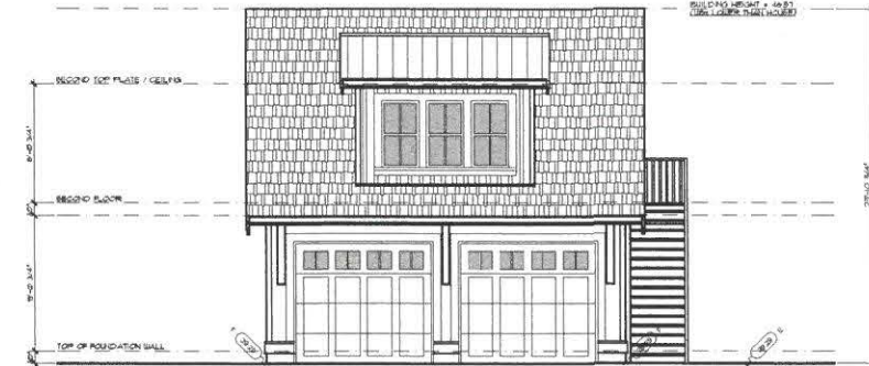
DETACHED GARAGE EAST ELEVATION SCALE: 1/4" = 1'-0"
